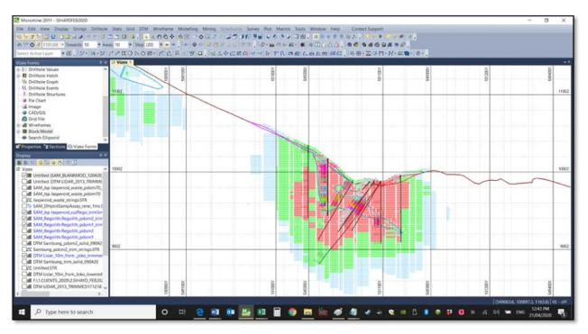
Figure 4-3. Figure 66: Sambung Sectional oblique view 3 of the block model displaying block resource categorisation
