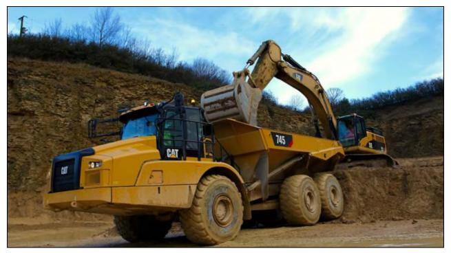
Figure 6-13. Cat 345 Excavator loading Cat 745 ADT
