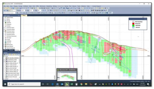
Figure 4-2. Sihayo Sectional view 54500mE of the block model displaying block resource categorisation (Figure 61).
