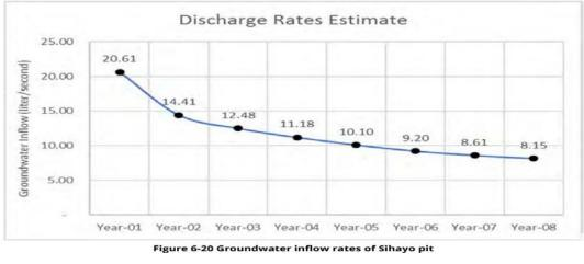
Figure 6-2. Groundwater Discharge Rates
