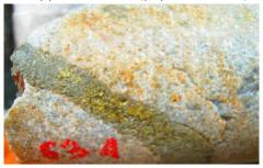
TTDD011 63.4m Quartz-pyrite-chalcopyrite veining in quartz-sericite-pyrite altered quartz diorite (62-64m: 3.04 g/t Au, 1310ppm Cu)
