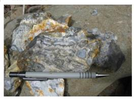
Hutabargot newly discovered "Fault Vein". Chalcedonic white quartz characterised by colloform banding and cockade textures
