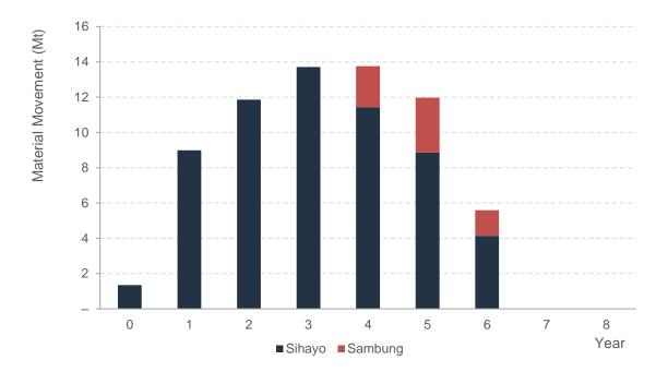
Figure A - 4: Project material movement schedule by deposit
