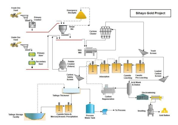
Figure A - 9: Process flow sheet
