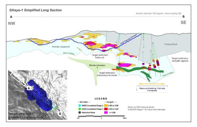
Figure 2: Schematic long section of Sihayo underground geology and Stage 1 & 2 drill hole traces
