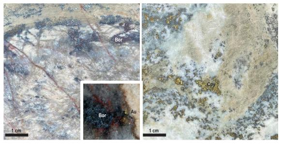
Note: Bor - bornite, Cpy - chalcopyrite, Au - free gold
