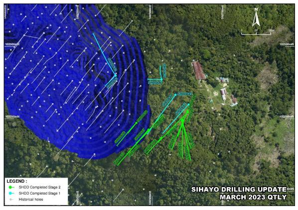
Figure 1: Stage 2 Sihayo Drilling Program – Drill Hole Locations
