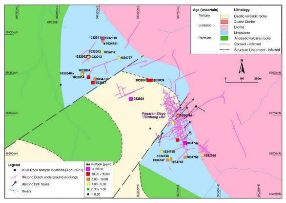
Figure 2: Tambang Ubi – Simplified Geology & Rock Chip Sample Locations (see Appendix 1 for complete list of samples and assay results)
