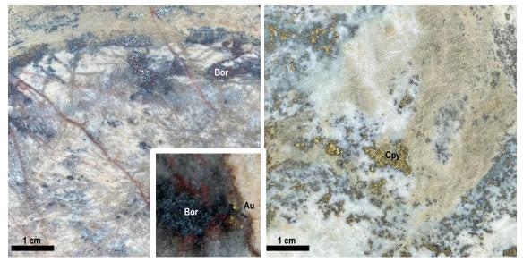
**Figure 3: Tambang Ubi – High grade gold-copper skarn samples** Bornite-rich (**Bor**) wollastonite skarn with free gold (**Au**) on LHS (Spl 1034744: 17.6 g/t Au & 0.93% Cu) Chlacopyrite-rich (**Cpy**) garnet-diopside-wollastonite skarn on RHS (Spl 1034746: 8.84 g/t Au & 3.38% Cu) (see Appendix 1 for complete list of samples and assay results)
