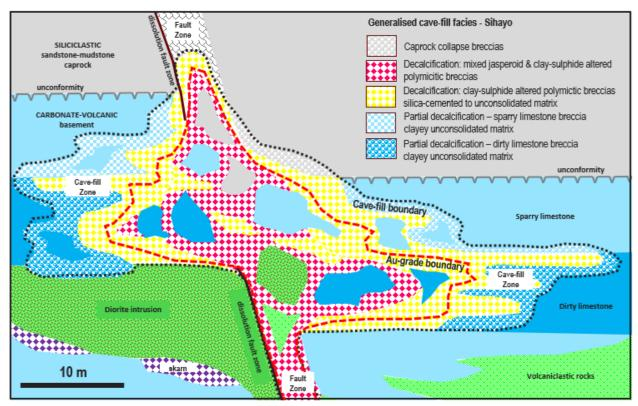
Generalised Schematic – Sihayo gold deposit A fault-controlled cave-fill mineralisation zone
