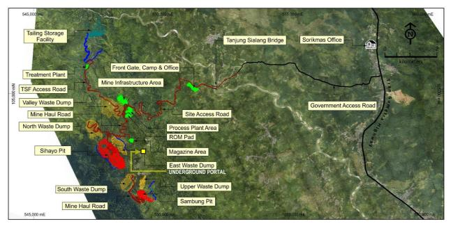
Figure 1: Sihayo 2022 FSU open-pit development layout plan
