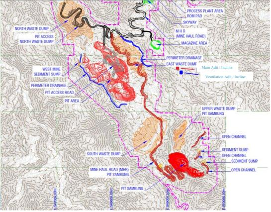
Figure 8: Surface Layout including location of Adits.
