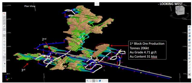
Figure 7: Looking west Sihayo underground mining 1<sup>st</sup> ore production.
