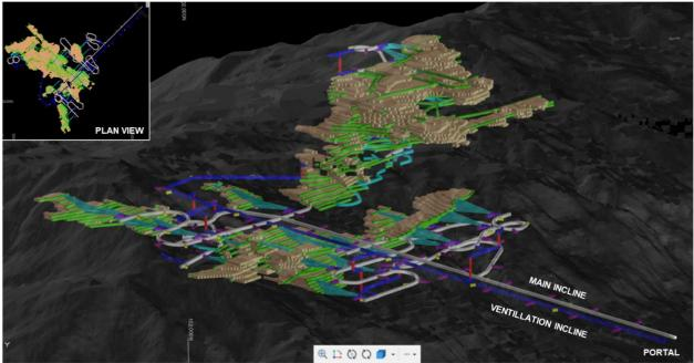
Figure 4: Sihayo Concept Study underground mine layout (Isometric view looking W) draped by LiDAR generated topography
