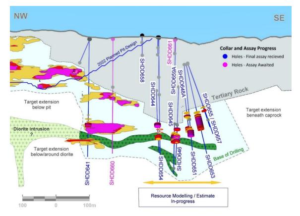
**Figure 1: Schematic long sections of Sihayo underground geology** Highlighting Stage 1 & 2 drill hole traces and position of reported intercepts (within a 25m envelope of the section line) Intercepts in holes SHDD656, SHDD658 & SHDD659a occur off section (See Figure 2)
